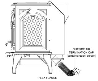
**NOTE:** If you plan to install the optional blower **and** the outside air kit, complete installation of the outside air kit **first**.
